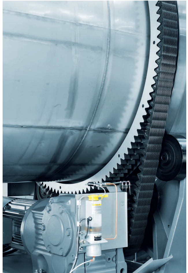
Tooth chain drive with automatic lubrication system
