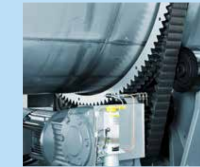
Toothed chain drive with automatic lubrication system
