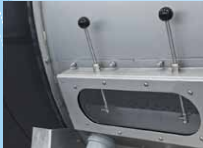
Wide overflow boxes for efficient lint removal.
