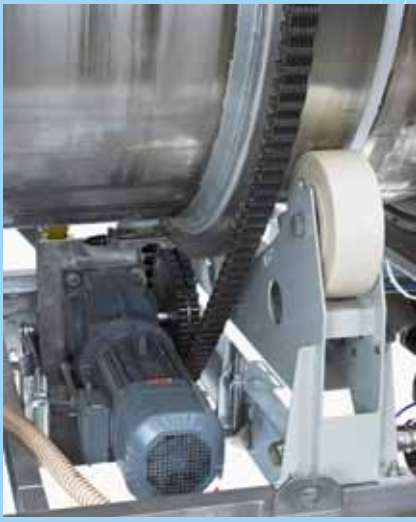
Drive unit with stable tooth chain.
