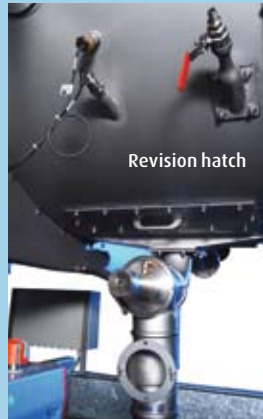
Drain valve with clamp closure and inspection window
